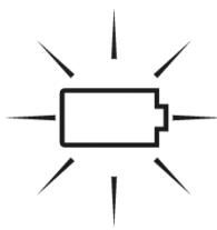
If the three bars on the display are blank and the outside frame flashes, the battery is flat and you must charge it. If you do not notice this, the device switches off automatically after a certain amount of time.
