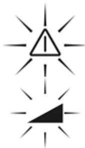
If external influences change the position of the device, the Autoslope monitoring system registers this and automatically initiates adjustment. If the device is tilted a relatively long way, the system interrupts rotation and the laser beam and the warning display flash rapidly.
